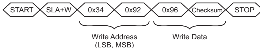
Figure 4-4. Example of a Write To Address 0x1234 With a Checksum
